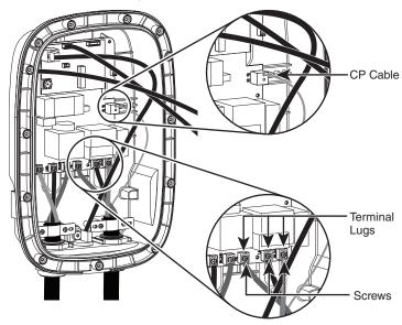
Tighten two screws securing clamping plate. Torque screws to 8.5 - 10.5 in-lb.
