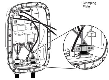
4. Loosen gland cap and remove cord.
