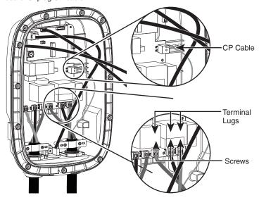
3. Loosen two screws on clamping plate.
