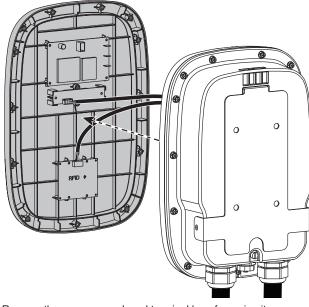
2. Remove three screws and cord terminal lugs from circuit board. Unplug CP cable.
