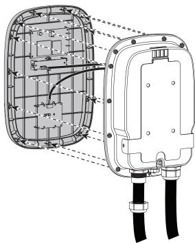
**5.** Tighten gland cap to seal. Torque gland cap to 8.5 - 10.5 in-lb.
