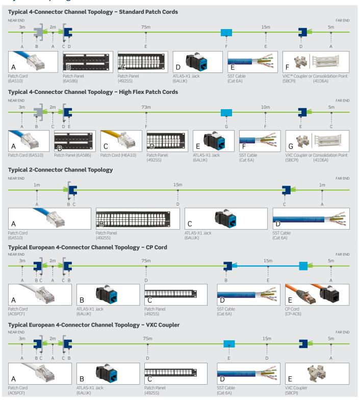
Note: Channels installed to support extended distance applications must have SST horizontal cable lengths that allow for a maximum of 10 m of patch cords and not exceed the maximum channel lengths shown in table 2 for the Ethernet speed and PoE power level to be supported.
