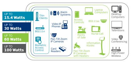
Both PoE tiers under the 802.3bt standard will support a range of enterprise devices, such as laptops and desktop computers, exterior-mounted IP cameras, information kiosks, industrial automation equipment, and next-generation wireless access points (WAPs). Publication of 802.3bt is anticipated for 04 of 2018.
