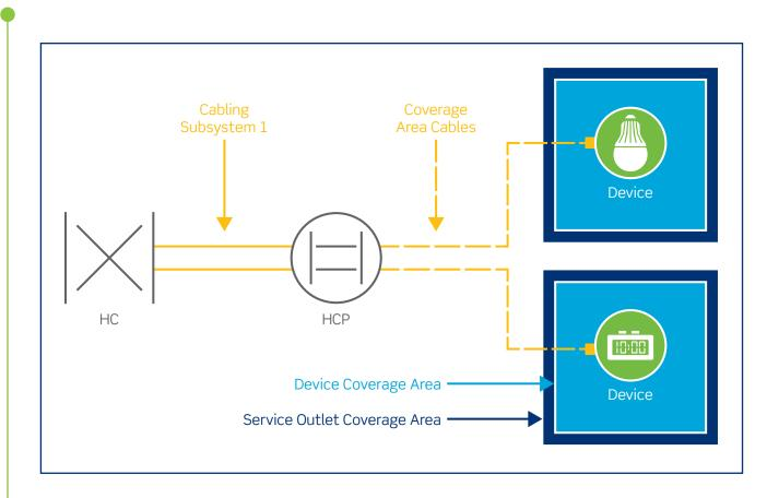
The best practice is to deploy horizontal cabling using a zone architecture where a Horizontal Connection Point (HCP) — essentially a consolidation point — services four to five Service Outlet coverage areas. Any HCP should be mounted permanently in an easily accessible area to allow for future moves, adds and changes.
