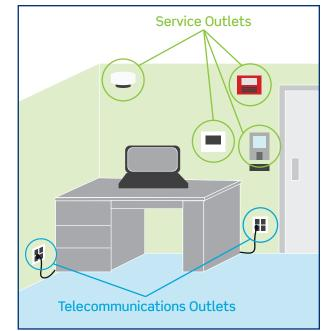
TIA 862-B assumes a service outlet coverage area of 3,600 square feet. Using this coverage area and anticipating the number of potential smart devices that could be needed, the recommendation is to plan for a minimum of 14 ports per service outlet coverage area, but optimally to install 18 ports per service outlet coverage area to allow for future growth.
