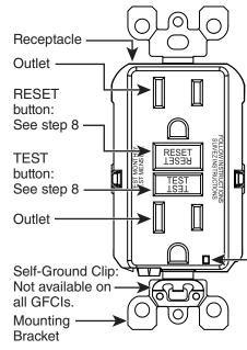
LINE Connection for the LINE cable's black wire.
